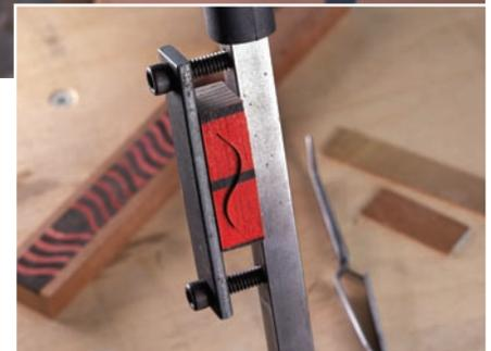
**That's money.** The cutters make this tool. Cut a wooden block to nearly any profile, affix a razor blade in between and you're ready to work.
